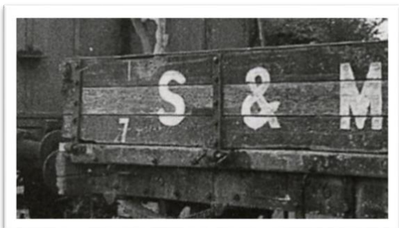
Later lettering style; S and R letters in outer panels & and M in centre. Numbers in LH corner. Wagon 9 however has prefix of 'No.' with small, underlined 'o' all in RH corner.
